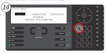
Once connected, the screen will display **STATUS**: **CONNECTED**.
