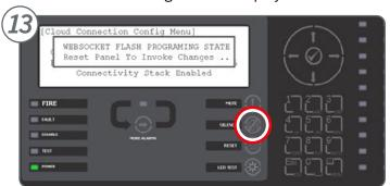
Press **RESET** button on the panel, Then wait for panel to reset and take you back to the main screen. (Repeat steps 1-4).
