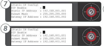
Use the **numeric keypad** to enter your IP address. In this example the IP address 192.168.001.123 is configured.
