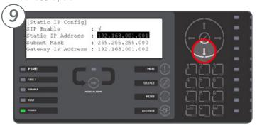
Once the IP address details have been entered, press the ESC button bottom/left of the numeric keypad, and then press [6] to select **SAVE CHANGES**.
