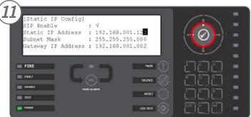
Press the **tick button** to accept the static IP address.
