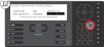
Press the **tick button** to display an **input cursor**.
