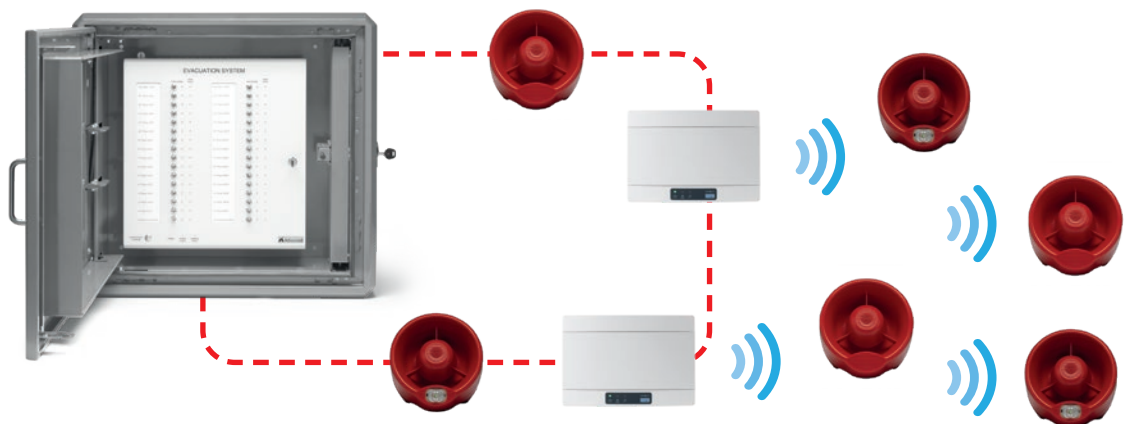
Example of hybrid evacuation alert system
